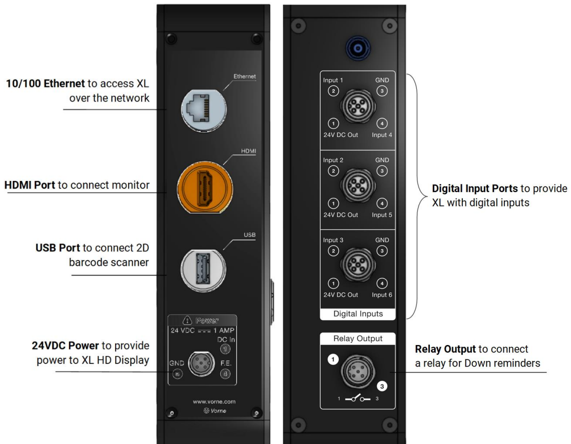
HD Side Views with Labeled Connections
